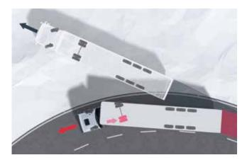
ESP compensatory braking when vehicle is understeered
